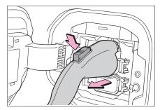
**3** Attach the charging connector cap.
