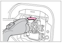
When the charging connector is inserted straight as far as possible, it will automatically lock.
