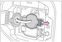
**5** Remove the charging connector cap and secure it to the cable.
