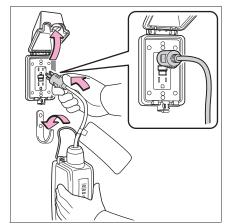
In order to reduce the load on the outlet and plug, when inserting the plug, use a string, etc., to hang the CCID (Charging Circuit Interrupting Device) on a hook or equivalent.
