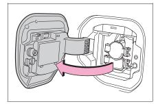
2 Open the AC charging inlet cap, and then open the DC charging inlet cap.
